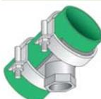
A quick and easy way to attach your pump's injection/check valve to your schedule 40 or 80 pipe, these clamp-on injector ports have 1/2" FNPT threads and are made of PVC with SS clamps.
