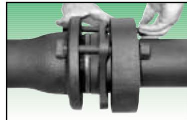
6. After the bolts are in place, remove the two T-head bolts holding the MJ gland and **BOLT-LOK** ring together. Discard the spacers which are used only for shipping. Reinsert the two bolts from the opposite direction and install the nuts.
