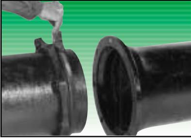
1. Clean the socket and the plain end. Lubrication is recommended for proper assembly of all mechanical joints. Lubrication and additional cleaning should be provided by brushing both the gasket and plain end with soapy water or pipe lubricant just prior to slipping the gasket onto the plain end for joint assembly. Place the gland on the plain end with the lip extension toward the plain end followed by the gasket with the narrow edge of the gasket toward the plain end.
