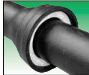
7. Insert the alloy steel locking ring into the groove. The ring may be forced into the groove if necessary. Once the ring is completely within the groove, the small wire-tie should be cut and removed. This will allow the locking ring to expand into place within the groove. This completes the **SNAP-LOK** assembly.
