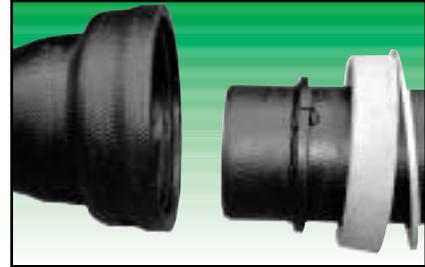
6. Slide the large **SNAP-LOK** restraining ring(s) fully into the bell socket. With proper insertion, the full depth of the locking ring groove should be visible. This is the groove closest to the face of the bell end.
