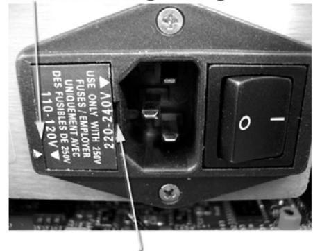
Insert a flat blade screwdriver to remove fuse cartridge Figure 11: Fuse
