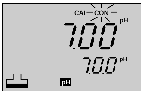
Figure 6 When you press YES to confirm calibration, the CON indicator blinks.
