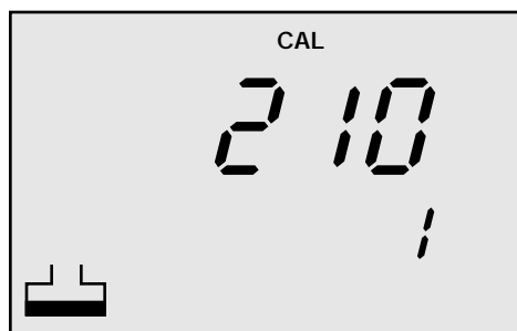
Figure 9 In Ion Calibration mode, the primary display (top) shows the ion concentration reading in mV and the secondary display (bottom) shows the number of the calibration point (1-5).
