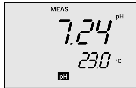
Figure 1 above shows primary display (here displaying pH) and secondary display (shows temperature).
