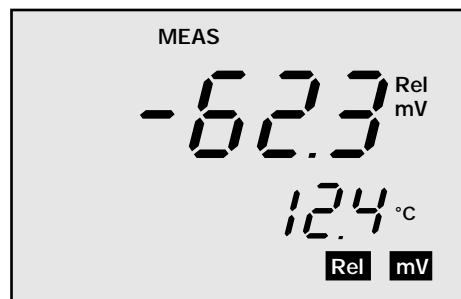
Figure 7 Upon entering the relative mV mode, the primary display shows either the relative mV value (if already calibrated) or the absolute mV value (if not calibrated yet). The secondary display shows temperature.
