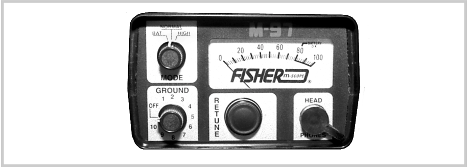
M-97 Control Panel
